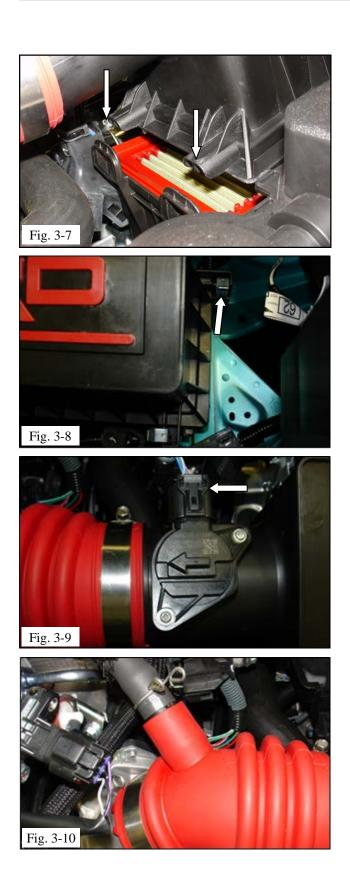
(g) Guide the inboard mounts of the air box top into the loops on the OEM lower air box (Fig. 3-7).
