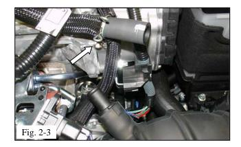
(c) Disconnect the crank case vent hose from the OEM air intake bellows, by pinching the spring clamp and pulling off (Fig. 2-3).
