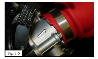
(f) Install the TRD coupler loosely on the throttle body (Fig 3-6).
