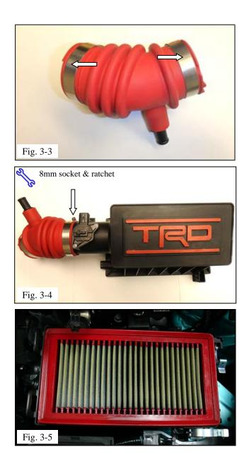
(c) On a workbench, install the 2 hose clamps loosely; do not tighten it at this time (Fig. 3-3).
